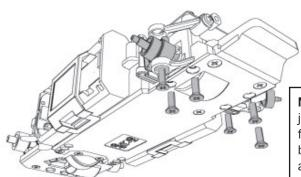
**Note:** Be sure the universal joints have not disengaged from the differential axles before screwing the assembly into place.
