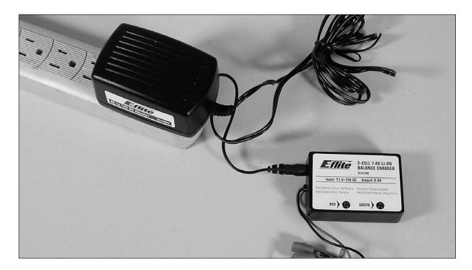
The charger is equipped with two LED indicators marked RED and GREEN on the label. These LEDs indicate the following (also found on the label of the charger):
