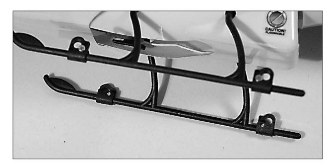
Locate the four training gear rods and rod mounting base. Note that the rod mounting base has four channels
