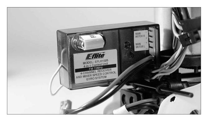
Turn the transmitter on first then plug the battery into the battery lead of the 4-in-1 unit.
