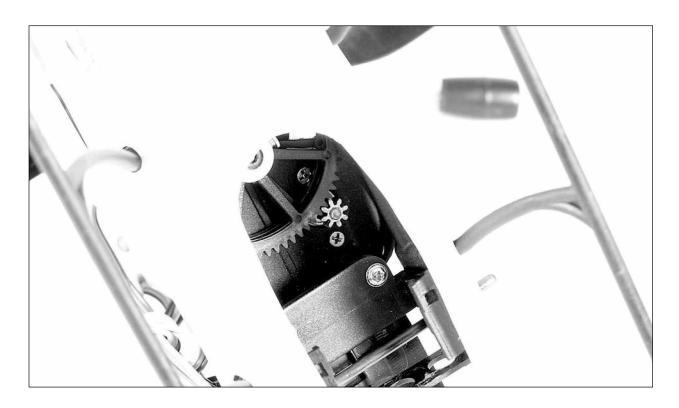
• With the right-hand main motor removed from the frame, you can press the main motor heat sink into place near the top/end of the left-hand main motor. We recommend that you use Heat Sink Compound (EFLM1913) on any surfaces of the heat sink that make contact with the motor case to further improve the effectiveness of the heat sink. The wider end of the heat sink (more fins) must be placed toward the front of the helicopter.
