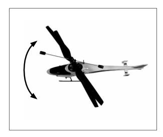
The right-hand stick controls both elevator (pitch fore/aft) and aileron (roll). Pushing the stick forward will pitch the nose of the helicopter downward, allowing the helicopter to be flown forward. Pulling the stick backward will pitch the tail of the helicopter downward, allowing the helicopter to be flown backward.
