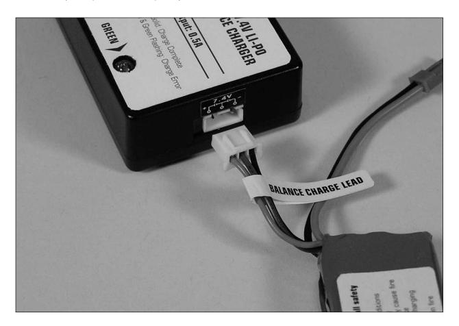
When the battery is properly connected and charging normally, the red and green LED indicators will glow solid. Once the battery has been fully charged, the green LED will go out, leaving just the red LED glowing solid. The battery can now be removed from the charger and installed into the Blade™ CX for flight.
