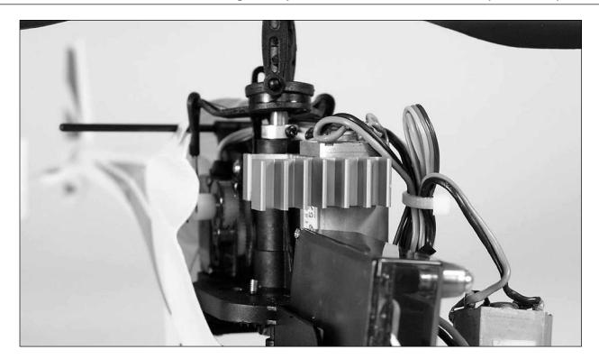
You can now press the right-hand main motor into place in the heat sink and use the motor mounting screws to
