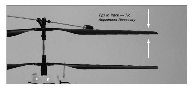
Typically, not much adjustment should be necessary to properly track the tips of the upper main rotor blade. However, due to the small size of the linkage ends and threaded rods it may not always be possible to achieve absolutely perfect blade tracking. Don't worry as the helicopter will still perform well as long as the blade tracking is adjusted as closely as possible.
